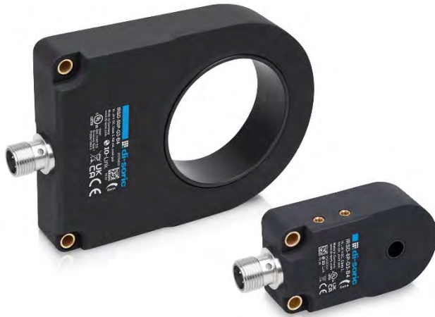
Image 1: From large to very small: the robust, multifunctional inductive ring sensors in the IRSD series by di-soric are available in 8 sizes with detection ranges between 6 mm and 50 mm.
