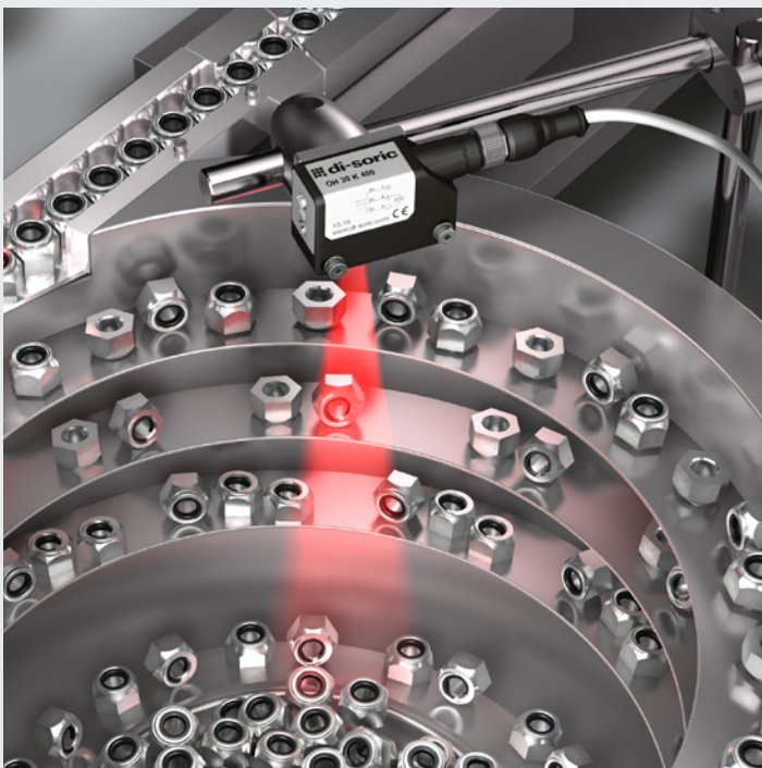
Optical sensor OH 30 K 400 P3-T4
