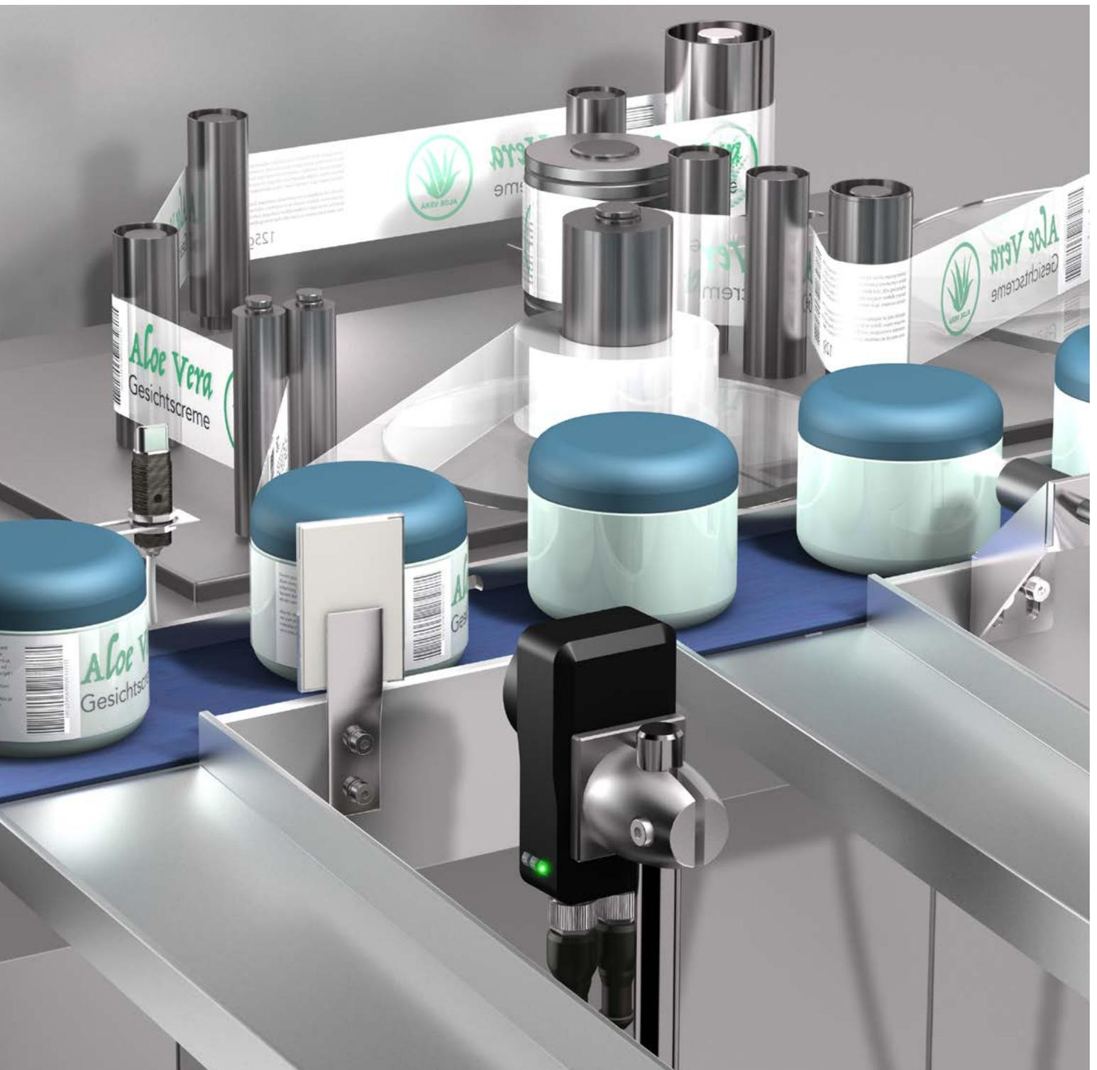
The ID reader in the rugged and compact IP67 housing is used in manufacturing companies in almost all industries. Strong algorithms ensure that all DPM codes are read, especially in the assembly & handling area. The IP67 protection class ensures that the ID-600 fixed-mounted ID reader works even in systems with high levels of dust, oil and dirt without any loss of performance.
