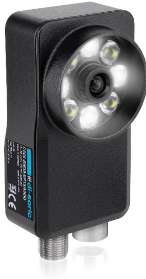
Image 1: Configurable CS-60 Vision Sensor from di-soric: with exchangeable M12 lenses and integrated LED high-performance lighting
